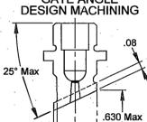
Nozzle body head must be keyed to prevent body from turning when tip is installed into body. Customer to torque (30±5 Ft Lbs) tip into shank of nozzle body in mold three times to set tip before marking the runner or angle on the tip. This will ensure that the tip will line up after runner or angle is machined onto tip. Customer may machine relief on Extended Sprue Gate and Extended Point Gate Tips for molding heat sensitive or engineering grade materials. (see drawings above)
