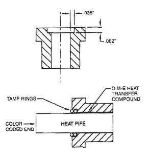
DME Heat Transfer Compound should be used when installing Heat pipe heat conductors. Take great care to avoid air pockets as air pockets are insulators that reduce heat transfer.
