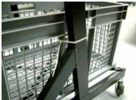
Attach Longer Cable Tie to Side Post
