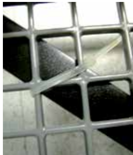
Attach Shorter Cable Ties to Corners
