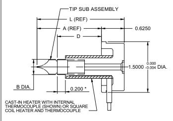
\* DIMENSION INDICATES CORRECT HEATER DISTANCE
