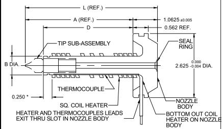
\* DIMENSION INDICATES CORRECT HEATER DISTANCE.
