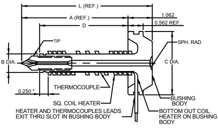
\* DIMENSION INDICATES CORRECT HEATER DISTANCE. Note: Dimensions shown in Inches.
